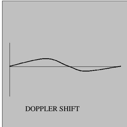
Figure 3. Control function for Doppler shift  $\frac{1}{D}$ .
